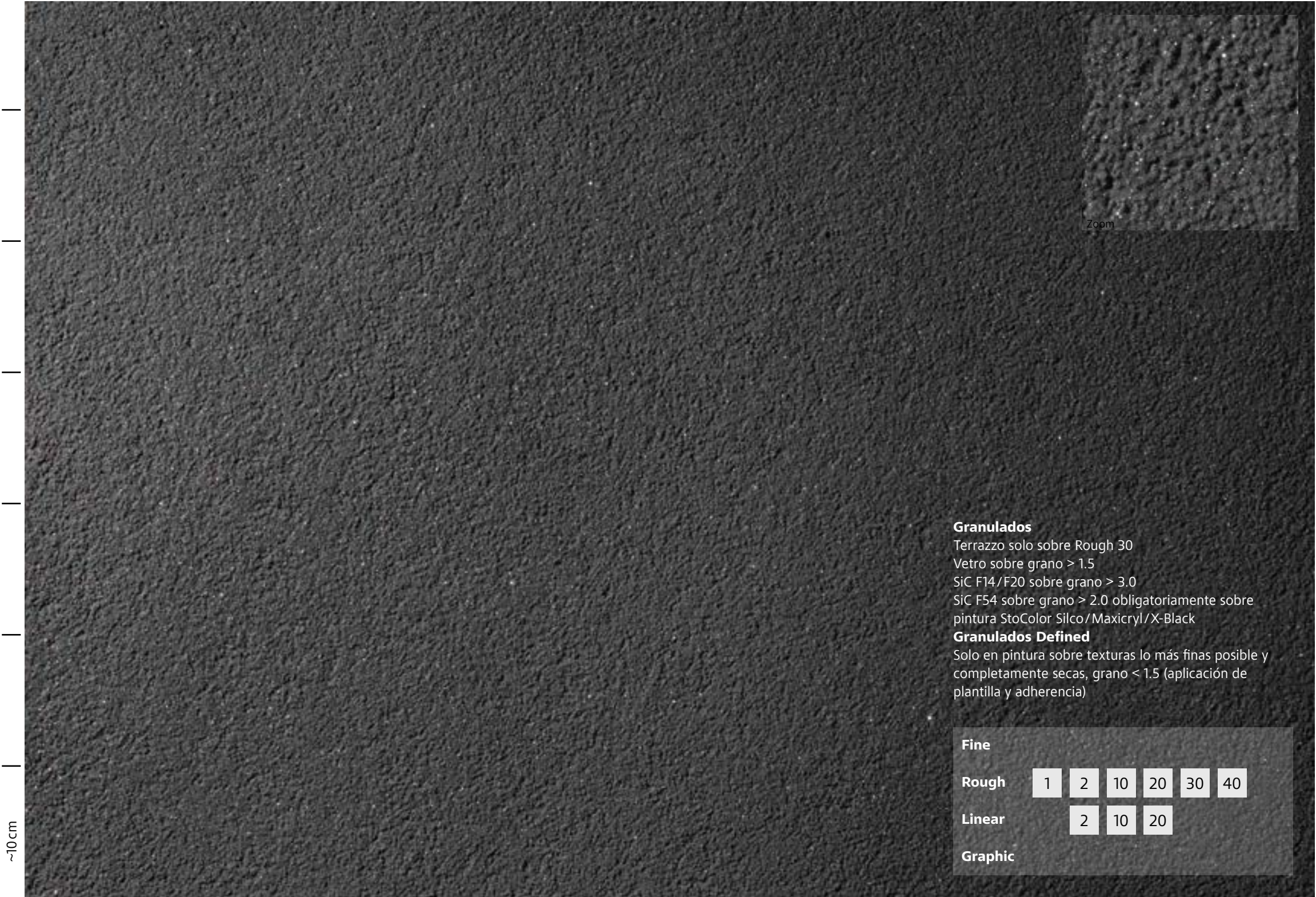
Textura: Rough 1, Stolit K 3.0 (37104) + Efecto: Granulate 30, StoColor Silco (37104)/Sto-Carburo de silicio F54
